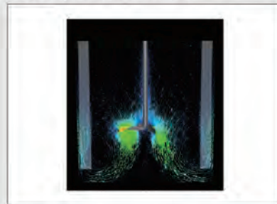
Fluid flow pattern in a stirred tank using HR320 impeller (C.F.D. Method)
